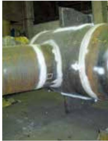
We tailor the vent silencers to the application in question and modify the dimensions and weight to offer the best possible solution. The strength of the pressure parts used for the silencers can be configured to meet common regulations inside and outside Germany. We have certified production facilities for ferritic, austenitic and martensitic materials (e.g. P 91).
