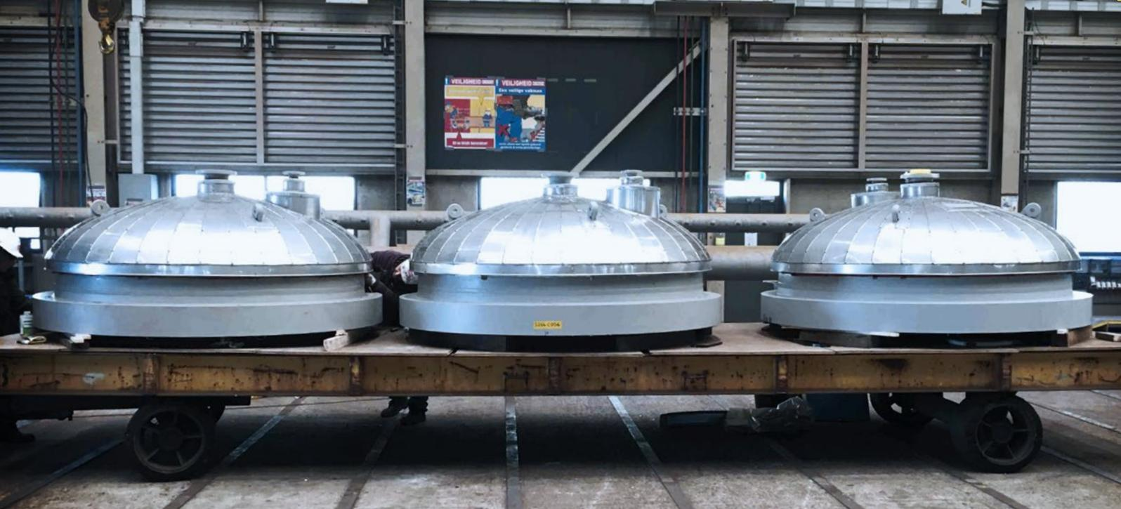
To prepare the pipes and containers of the new offshore rig for the rough conditions at sea, G+H Insulation applied a special multi-layer installation method. First the team fastened two layers of 19 mm Armaflex all around, using adhesive, and then surrounded it with a 1 mm flexible Arma-Chek film, sealing the seams with Mastic. The outer coating took the form of 0.6 mm stainless
